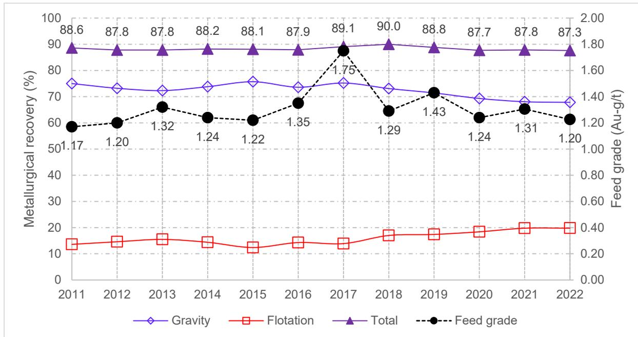
Figure 13-1: Plant Recovery and Feed Grade Data 2011 to 2022
