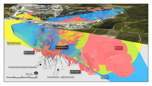
Figure 1: Perspective view of the Björkdal Mine looking towards the SSW highlighting the interaction of the veining (Red) Marble (Blue) and Björkdal fault (Yellow). Drilling of the latest Central Zone extension programs is also shown.
